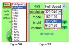
NOTE: You can reduce file size by setting the resolution lower, as in figure 3.9.
